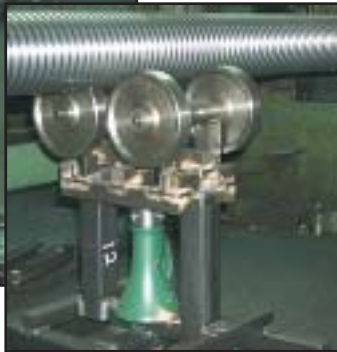
Simplex screw jacks are used to adjust the height of this roller fixture. "We use this fixture during the assembly of long pieces of screw stock." "Simplex screw jacks makes fixturing easy and precise."
