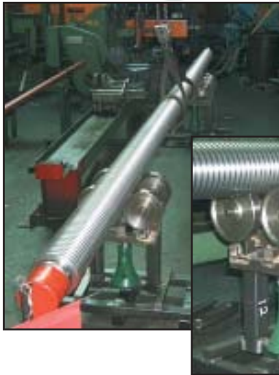
Simplex screw jacks are used to adjust the height of this roller fixture. "We use this fixture during the assembly of long pieces of screw stock." "Simplex screw jacks makes fixturing easy and precise."
